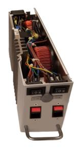
In Power Through (BP-Constant) Mode the circuit will completely bypass the Choke and SSR giving you clean power to your Lighting devices and power supplies that require a constant power feed. In Non-Dim Mode (ND) the delivery of full power to the load is controlled via the Console.
