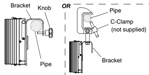
\* Mounts to 1.5" Schedule 40 pipe or 2" aluminum tube truss.
