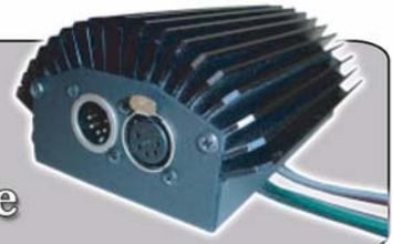
The Light Pack IGBT Dimming Module can be mounted in a variety of configurations. Depending on your requirements, choose one of the methods shown below. The module can be mounted vertically (recommended) or horizontally as required, however, to allow for optimum convection cooling, it CANNOT be mounted with the heatsink fins downward.
